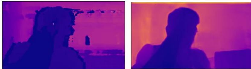
Figure 4.1: Left image: depth map estimated by OAK-D; Right image: depth map estimated by the Monocular Depth Estimation
