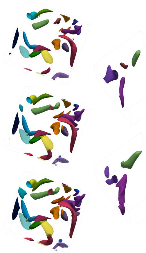
Figure 8: To track features in the turbulent vortex data, we compare the complete extremum graphs of consecutive time steps. Tracked features across time steps 2, 4 and 6 are shown on the left. Low opacity values indicate higher structural distortion in the complete extremum graph. Three features are shown in isolation on the right, the violet feature undergoes a split. The green and brown features merge, the purple feature grows.
