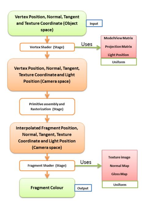
Figure 4.13: Programmable graphics pipeline
