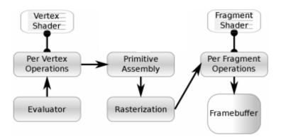
Figure 3.4: Stages of programmable graphics pipeline.
