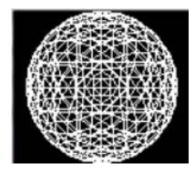
Figure 3.1: Triangular mesh for a sphere.
