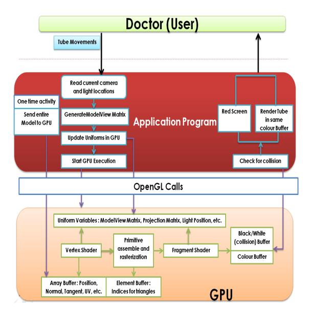
Figure C.1: Internal working of graphics system
