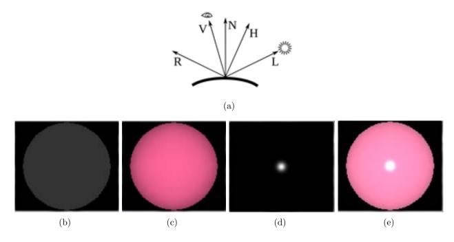
Figure 3.2: Lighting and shading demonstrated on a sphere. (b) A sphere with only ambient lighting. (c) Same sphere with only diffuse lighting. (d) With only specular lighting. (e) The combined effect of all three lighting. (a) The vectors involved in lighting calculation. L is light vector, V is viewing vector, N is normal to the surface, R is reflection vector, while H is halfway vector between V and L.
