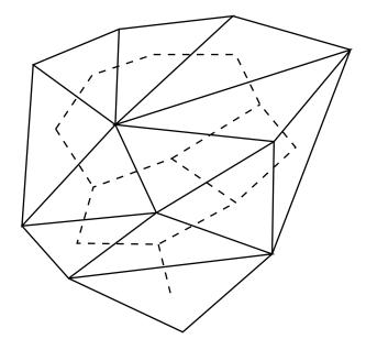
Figure 4.4: A triangle mesh (solid line) and its dual graph (dotted lines).
