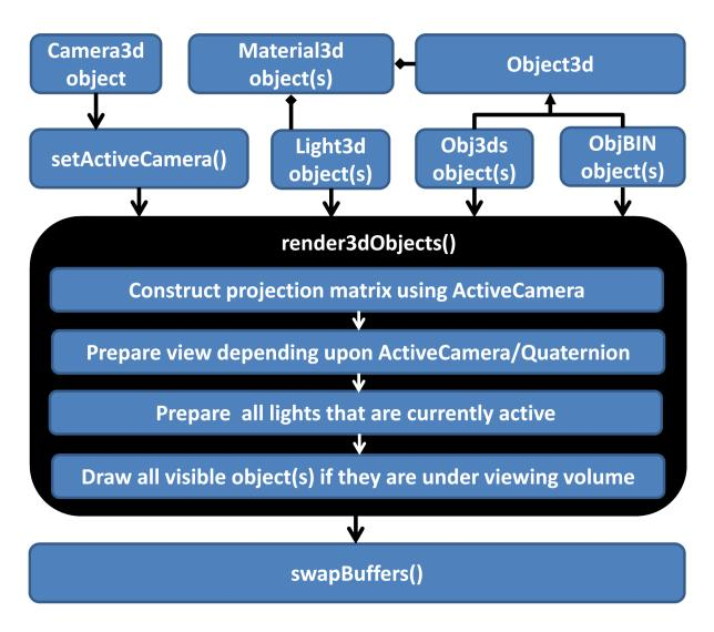
Figure A.2: Internal working of 3D engine
