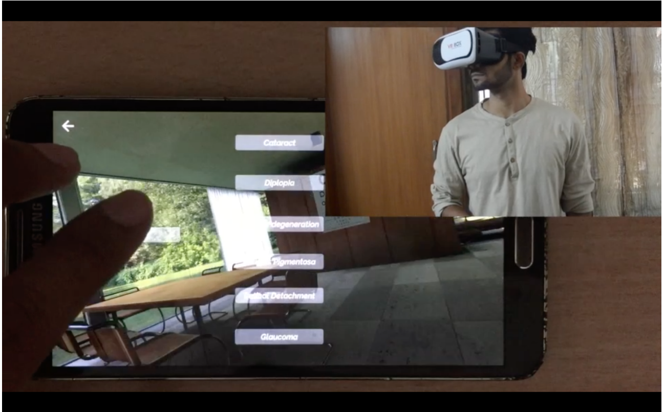
Figure 1.1: UI of EmpathEyes shows monoscopic view on the phone screen along with a list of presets for some of the simulated impairments, inset shows the immersed user wearing a Google cardboard
