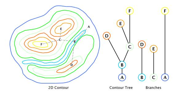
Figure 3.1: A terrain with contours (right picture) representing a 2D scalar field; The critical points are: A is minima, B and C are saddles, D, E and F are maxima; The graph on the right shows how the contours begins from A, splits at B and C, and finally ends at D, E and F. The contour tree and branches for the scalar field in the middle and right respectively.
