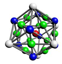
Figure 5.7: 26 points based neighborhood due to Face-Centered 24-fold subdivision. The navy blue colored spheres are body-centered points; green colored spheres are face-centered points; white sphere are the original points; the internal red sphere is the original point in contention for classification.
