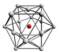
Figure 4.2: 18-points based neighborhood marked as white spheres; their connectivity is shown using grey edges; surrounded red sphere is in contention for classification.
