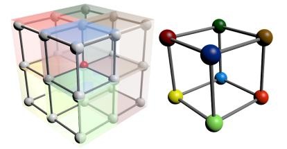
Figure 5.3: The 26 neighboring points around a subsampled point with the neighborhood set formation for each of 8 points in the locality
