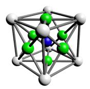
Figure 5.10: The neighborhood structure for a body-centered point point of size 14
