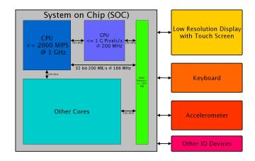
Figure 2.1: Diagram of a sample System on Chip (SOC) used in mobile devices
