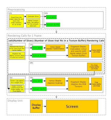
Figure 2.2: Volume rendering pipeline used in our implementation
