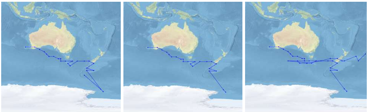
Figure 3.5: Sensitivity analysis of the clustering threshold. Representative tracks over the Australian bay area during May 1994 computed with constant isovalue threshold of 0.45. (a) Clustering threshold is set to 20. A small split is visible close to lysis. The two proximal sections of the tracks are not clustered together. (b) Representative track for clustering threshold equal to 44, as identified from the plot in Figure 3.4. This track, and its lysis, is physically more plausible, because large jumps of the cyclone track towards the west are highly unusual since the prevailing winds in this region are towards the east. Varying the clustering threshold between 40-50 has no effect on the representative track. This indicates stability of the selected clustering threshold. (c) Increasing the clustering threshold to 60 results in remote tracks to be clustered together.
