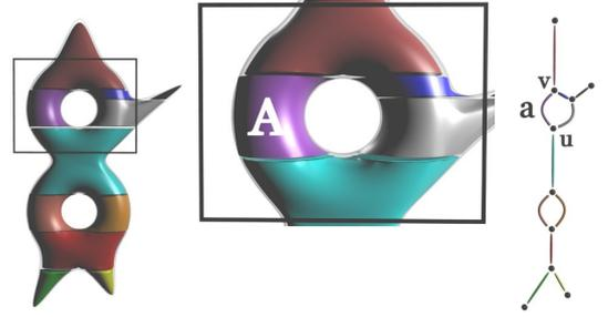
Fig. 2. Reeb graph of the height function defined on a solid 2-torus. The Reeb graph tracks the topology of level sets. Arc  $a$  in the Reeb graph maps to cylinder  $A$ , a collection of level set components.
