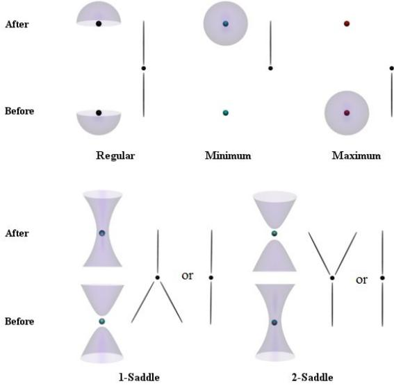
Fig. 1. Isosurfaces before ( $f^{-1}(c - \epsilon)$ ) and after ( $f^{-1}(c + \epsilon)$ ) passing through a point with function value  $c$  and the structure of the Reeb graph at the corresponding node. Topology of the isosurface changes when it evolves past a critical point. Genus modifying saddles and regular points are optionally included into the Reeb graph as degree two nodes.
