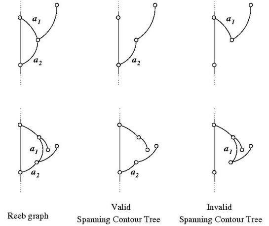
Fig. 9. The spanning contour tree of a Reeb graph is structurally similar to a contour tree. Removal of  $a_1$  results in a spanning contour tree. Removing  $a_2$  results in a tree with an invalid degree-2 node.
