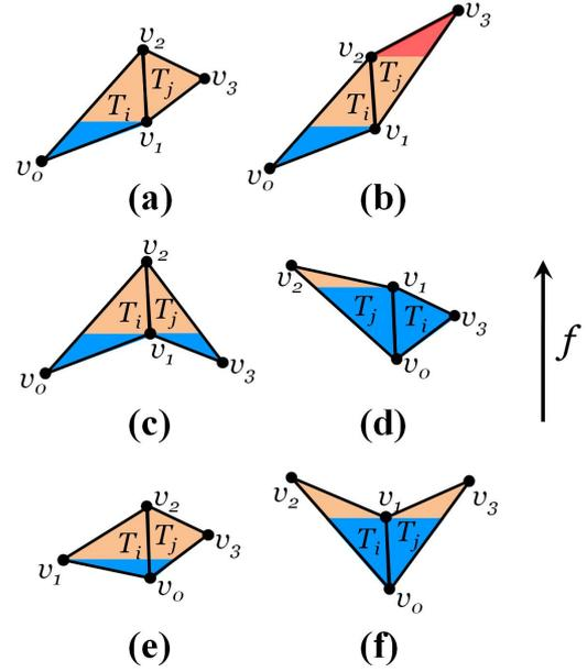
Fig. 3. Adjacent triangles in the input can have one of six possible configurations. The *LS*-graph contains an edge from  $t_i$  to  $t_j$  in all cases except the forbidden configuration in (f). Edges in the graph are directed towards the node with higher cost. The boundary between the blue and orange regions and the boundary between the orange and red regions indicate the location of the level set edges where the function value becomes greater than  $f(v_1)$  and  $f(v_2)$  respectively.
