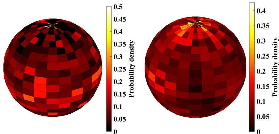
Fig. 13: (left) Normalized particle stereographic histogram and (right) normalized contact spherical histogram for sand packing.
