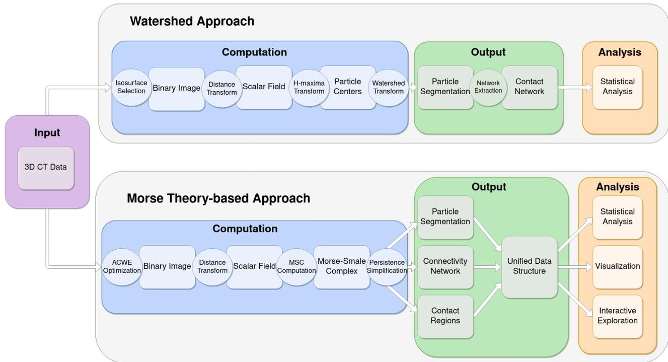
Fig. 1: Visual comparison of the watershed-based and the proposed Morse theory-based approaches to process and analyze 3D CT data. The comparison helps identify key differences between the two method pipelines in terms of computation, output, and supported analysis. The unified data structure retrieved from the MS complex supports various analysis tasks.
