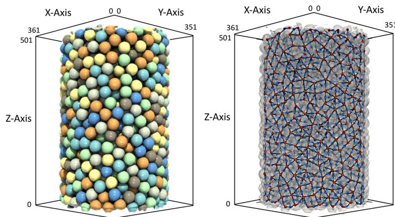
Fig. 7: The segmentation (left) and connectivity network (right) for the mono-dispersed steel bead packing.
