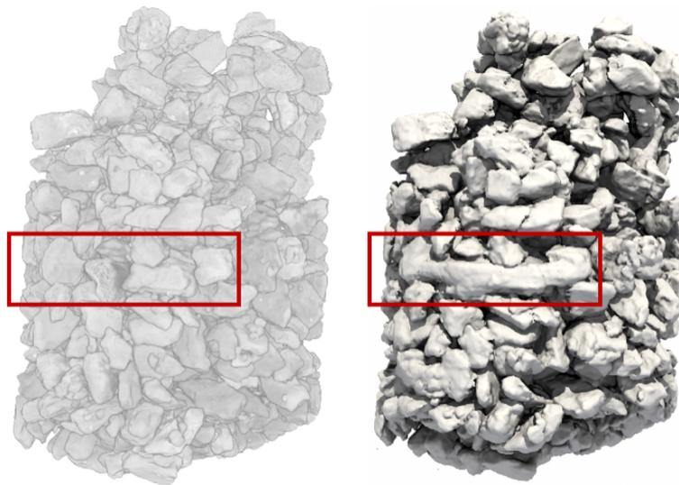
Fig. 3: Left: Direct volume rendering of the CT data using a fine-tuned color map. Right: Manually selected isosurface guided by a histogram. Notice how the isosurface does not agree well with the CT data, specially in the region enclosed by the red box.
