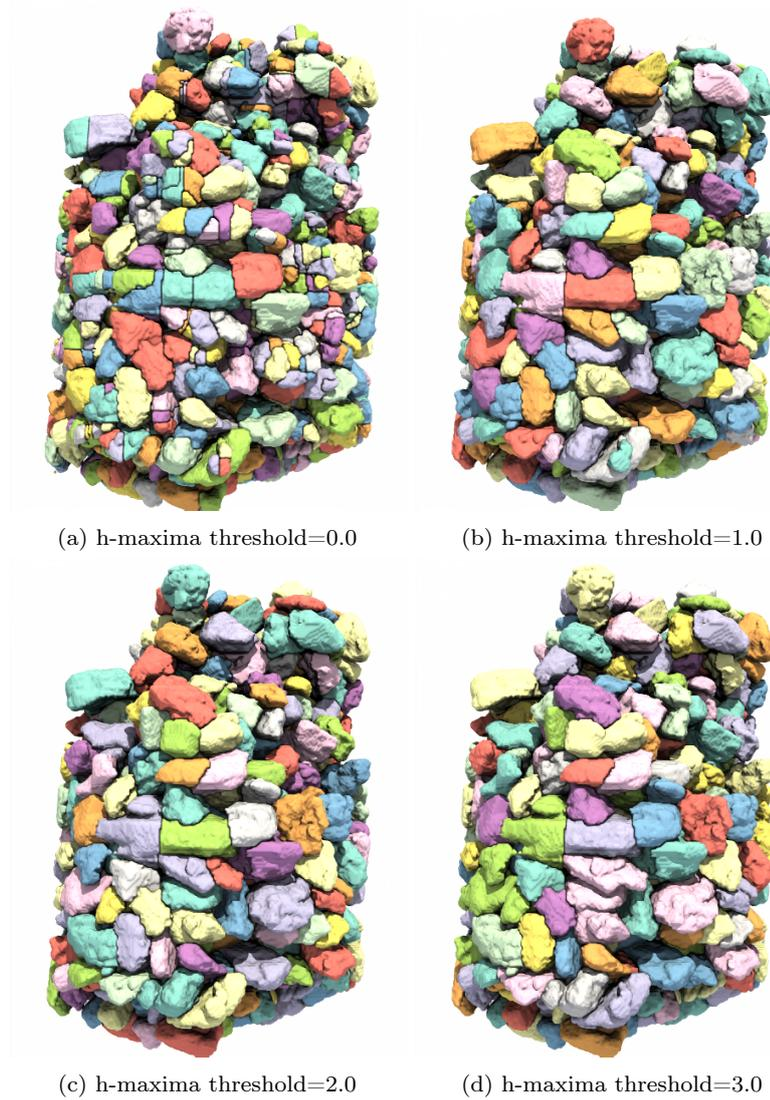
Fig. 4: In the watershed-based approach to segmentation, it is challenging to identify a “correct” h-maxima threshold. Note how the chosen threshold affects the final segmentation. Often, this threshold is chosen using a trial-and-error process. In some cases, the threshold identification is guided by prior knowledge of the sample, say the expected particle size or expected number of particles in the sample.
