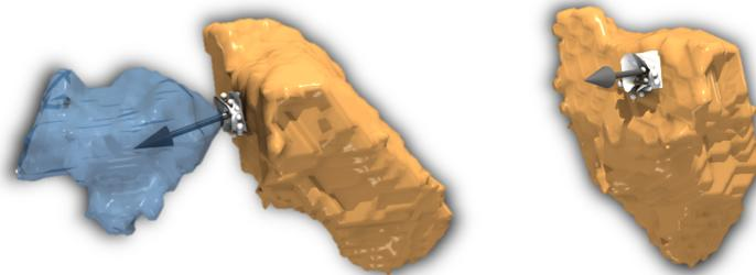
Fig. 10: Extracted region and orientation of contact between two sand particles colored in blue and brown. The translucent gray surface represents a clip of the extracted boundary surface of the particles near the contact region. This surface is the descending 2-manifold of the 2-saddle that defines the contact. Constituent points of the contact region are represented as white spheres, with the arrow displaying a fitted normal vector to the contact.
