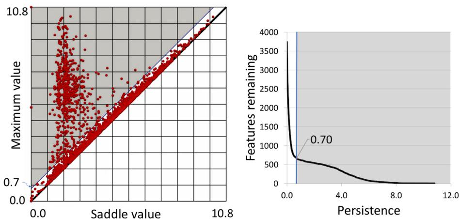
Fig. 11: Persistence diagram (left) and curve (right) for the cemented sand packing. The knee in the persistence curve (0.7) informs the choice of a noise threshold that separates features from noise. We can see how the selected threshold removes the cluster of low-persistence noise (white region) from the remaining features (grey region) in the persistence diagram.
