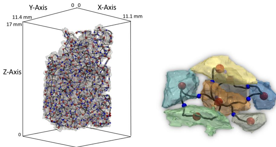
Fig. 9: Global (left) and local (right) visualization of the geometric embedding of the extracted connectivity network of the packing. In the local view (right), bead centres are represented as red spheres and contacts as blue spheres.
