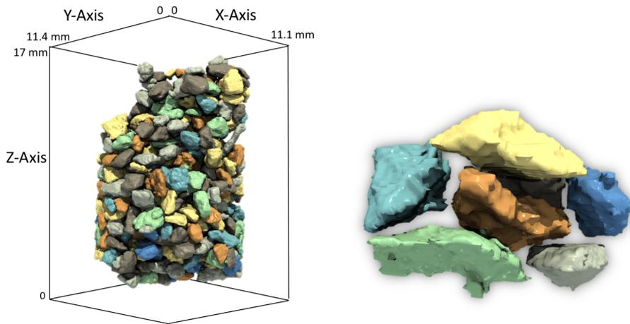
Fig. 8: Global (left) and local (right) visualization of the segmentation of the packing into its constituent individual particles. Particles are colored by their segmentation identifiers.
