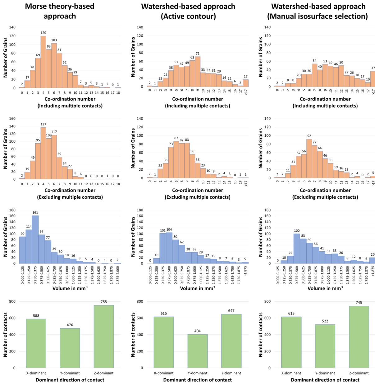
Fig. 12: Statistical analysis of sand granular ensemble computed using the Morse theory-based and watershed-based methods. Histogram of coordination numbers is similar when counting contacts with multiplicity, else the histograms are similar. The distribution of volume of particles is similar but the actual counts are different.
