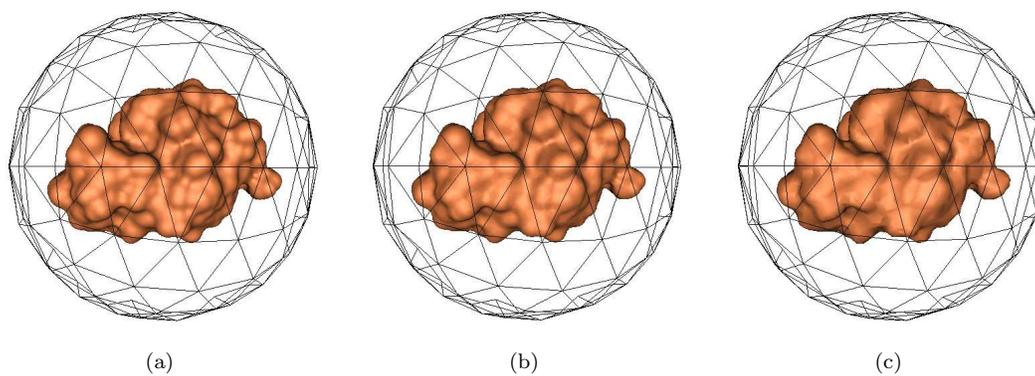
Figure 6.2: Molecular surface simplification. The mesh representing the volume occupied by the protein molecule (PDB ID: 193L) is simplified while preserving the topology of the molecular surface. From left to right - molecular surface at 100%, 30% and 10% of original data.
