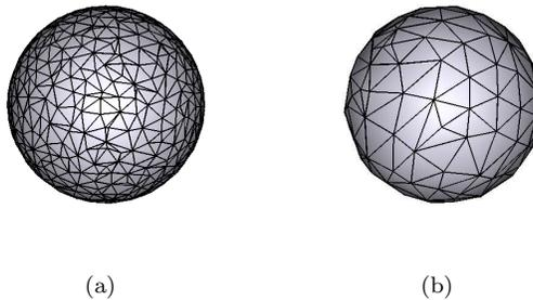
Figure 2.2: (a) Embedded structure before and (b) after simplification.
