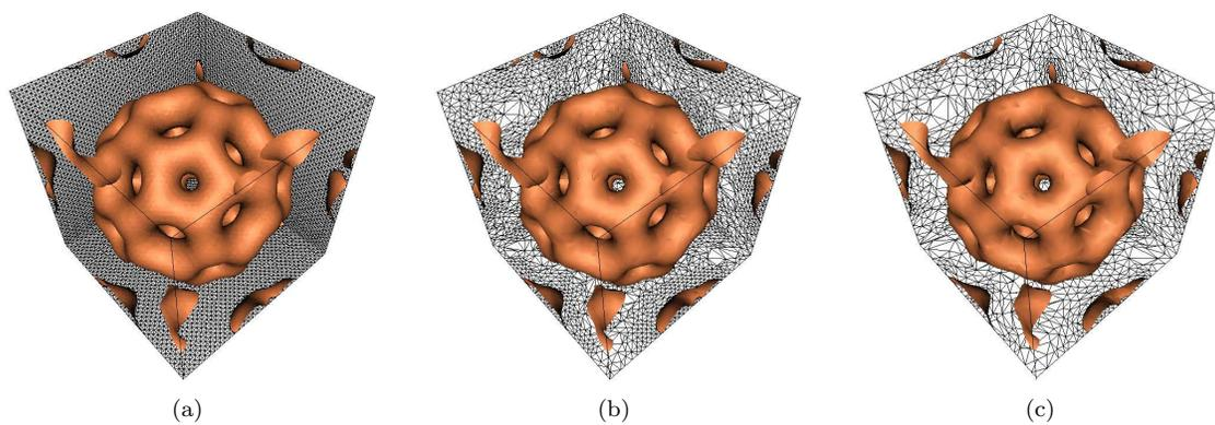
Figure 6.1: Isosurface topology preserving volume simplification. From left to right - isosurface at 100%, 30% and 10% of original data.
