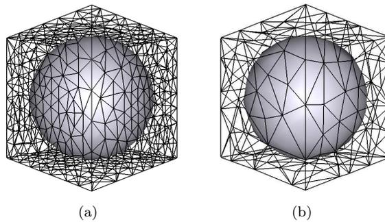
Figure 2.1: (a) Original and (b) simplified volume containing embedded structure shown in grey.
