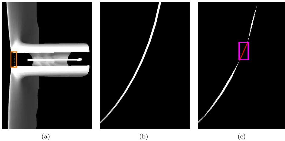
Figure 7.1: Topology violation of embedded structure. (a) Embedded structure with a ring like portion. (b) Magnified view of the ring like portion which is a 2-manifold with boundary. (c) After simplification, a principal edge appears (shown in red) and violates topology.
